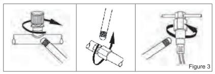
Sensor tip must be installed before any testing and detecting occur. Make sure the power is turned off. Use the tip come with detector or authorized replacement tip only. Line up the thread on the sensor tip with flexible probe end crew, turn it clock-wise and hand tight only.
