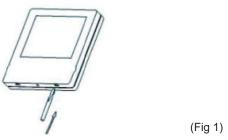
1. Open the control board by a Flat-blade screwdriver in the position of Fig 1.
