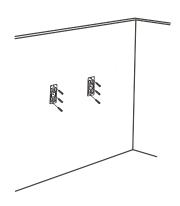
4. Fix on the wall with expansion screws.
