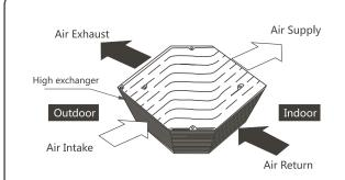
Energy saving during air exchange Effectively recover the energy lost due to ventilation.
